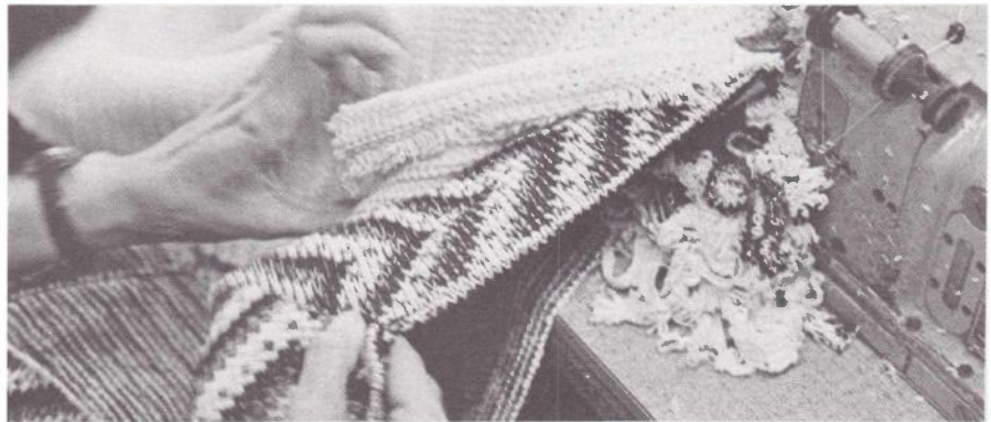
Border treatments have become one of the more common styling details in Roosevelt's knitted outerwear. Above, operator stitches border to body. Below, she turns the already prepared border corner before continuing.
