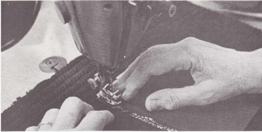
First step in making welt pockets like those on cardigan at right, is the stitching down of the welt/interlining portion on garment face, above. After other pocket piece is sewn, operator cuts slit between, below.
