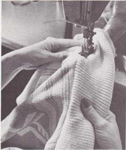
Overlock stitch is applied by operator to seam where collar is joined with wrap cardigan body.
