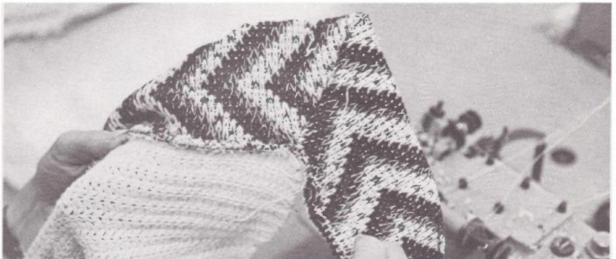
Border treatments have become one of the more common styling details in Roosevelt's knitted outerwear. Above, operator stitches border to body. Below, she turns the already prepared border corner before continuing.
